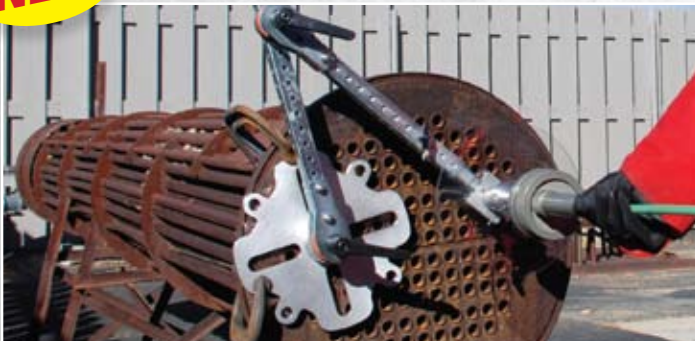
VE 400™ Backout Preventer for safe flex lancing.
